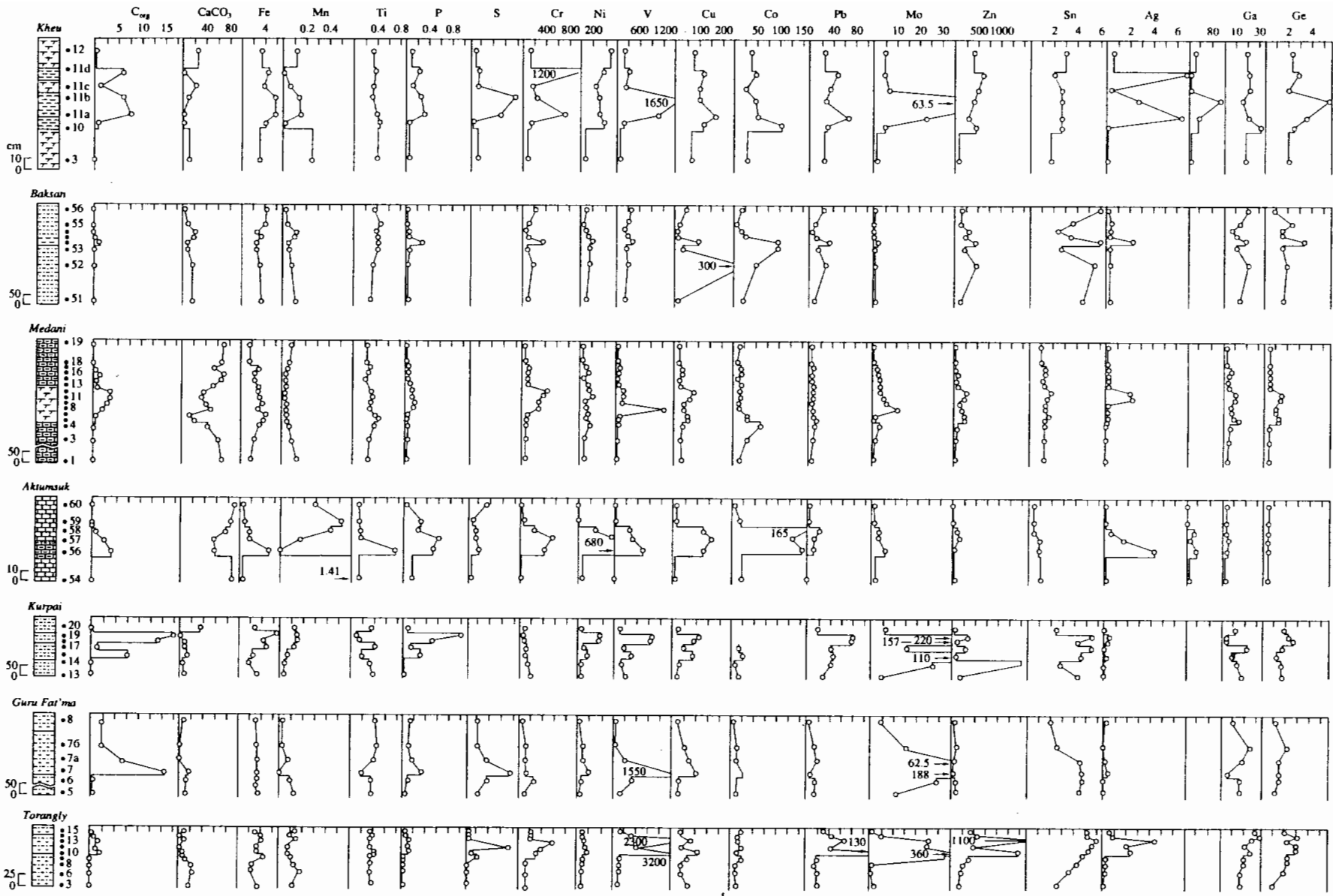
Fig. 3. Distribution of chemical elements in the sapropelite unit sections. C org , CaCO 3 , P, Ti, Fe, Mn, and S are given in %; other elements, in ppm. (1) Shales; (2) silt clays; (3) siltstones; (4) marl clays; (5) marls; (6) limestones.
