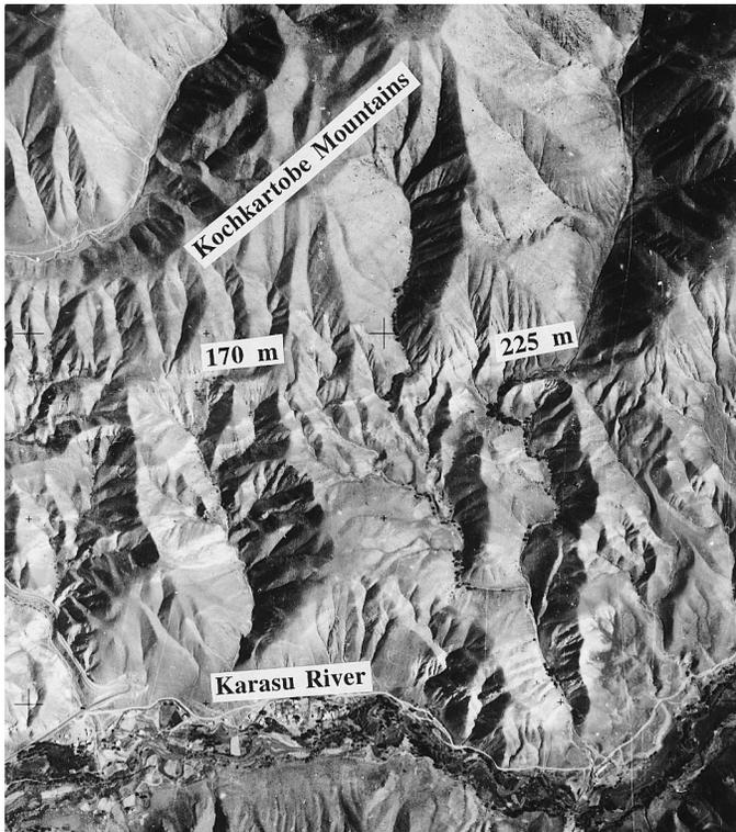
Figure 20. Aerial photograph of the Talas-Ferghana fault near the Karasu River. Two offsets, one of  $\approx 225$  m (see Fig. 19) and another of 170 m, are marked.
