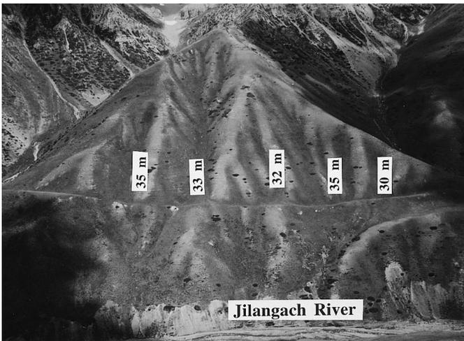
Figure 7. Photograph, using a lens with a focal length of 20 mm, looking northeast at the trace of the Talas-Ferghana fault on the hillside across the Jilangach River. After measuring one distance with a tape measure, we estimated the offsets shown by scaling them by eye. Most offsets are estimated to be  $\approx 30\text{--}35$  m. This area is  $\approx 5.5$  km southeast of Jilangach Pass.
