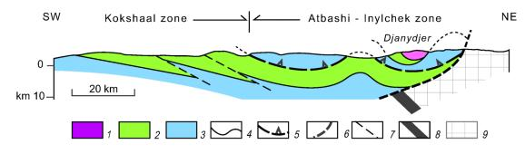
**Figure 16.** Units of the Atbashi-Inylchek and Kokshaal tectonic zones in geologic section along the line A in Figure 15. 1–3 – Units: 1 – Keltubek and Inylchek, 2 – Chatyrkul and Maidantag, 3 – Kokkiya and Muzduk; 4 – Primary overthrust faults; 5 – Borkoldoi secondary overthrust fault; 6 – Atbashi-Inylchek fault; 7 – Other faults; 8 – Turkestan oceanic suture; 9 – North Turkestan domain. *Djanydjer* – Djanydjer synform.
